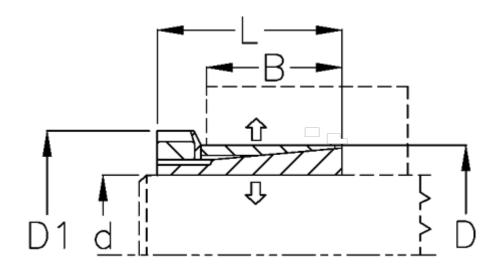
$\begin{array}{lll} \text{B mm} & = 17 \\ \text{D1 mm} & = 32 \\ \text{d H8 mm} & = 16 \\ \text{D mm} & = 25 \\ \text{Fit tolerance} & = \text{Aksel h8, Nav H8} \\ \text{F kN torque} & = 12 \\ \text{L mm} & = 29 \\ \text{P N/mm2 surface pressure on shaft/hub} = 60 \\ \end{array}$
